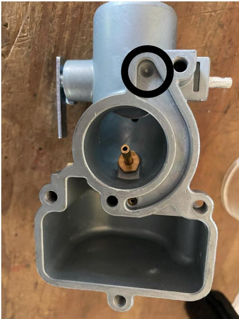
If the hole is not drilled completely through, as shown in the image, it should be. You have two choices. You can return the carburetor to the seller and demand a properly completed unit. Or, you can finish drilling the hole yourself, using an 11/64 bit. Be careful not to drill too far, damaging the rest of the part.
